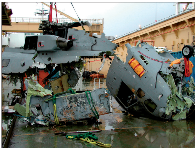
Figure 11: EH 101 Merlin ditched. The aircraft was on fire at time of impact. Note failure of inflation bags to activate. Each bag represents over 3 tonnes of positive buoyancy and a massive risk to operators during recovery.
