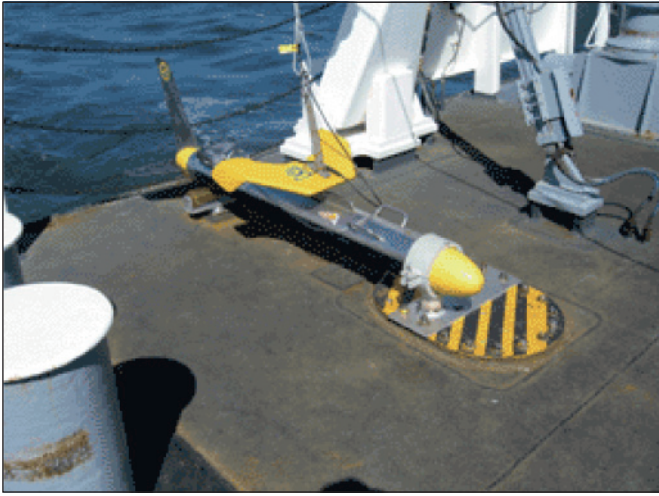
Figure 5: Typical side scan 'fish' rigged for deployment over the stern. The image does not show the handling winch, launch array or the control cab also required to operate the system.
