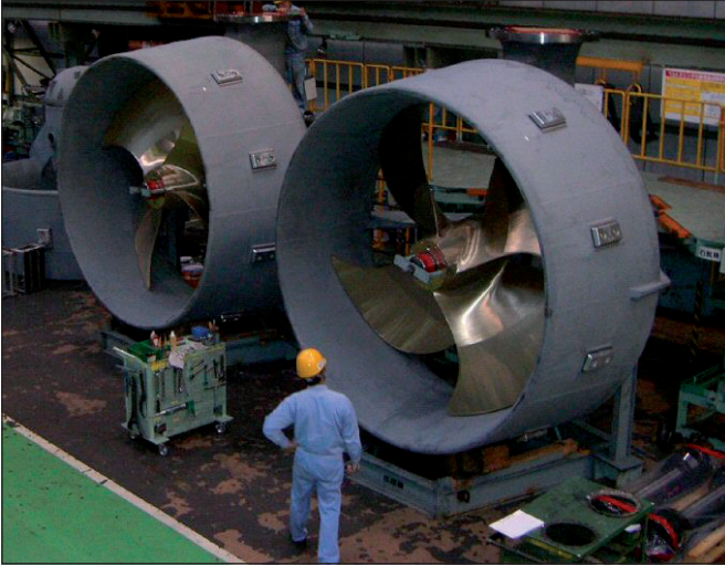
Figure 19: New design ducted propeller at full-scale.
