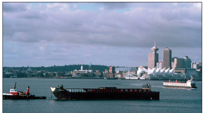
Figure 10: Empty limerock deck cargo barge (10,000T dwt) in Vancouver Harbour.
