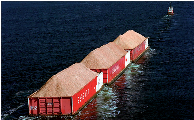
Figure 4: Triple tow of chip barges in Howe Sound near Vancouver. Barges are connected with short nylon 'couplers'.
