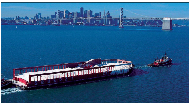
Figure 6: Large bulk cargo barges are commonly used for products such as salt (illustrated), gravel, limerock and stone. Some are equipped with built-in hoppers for cargo discharge.
