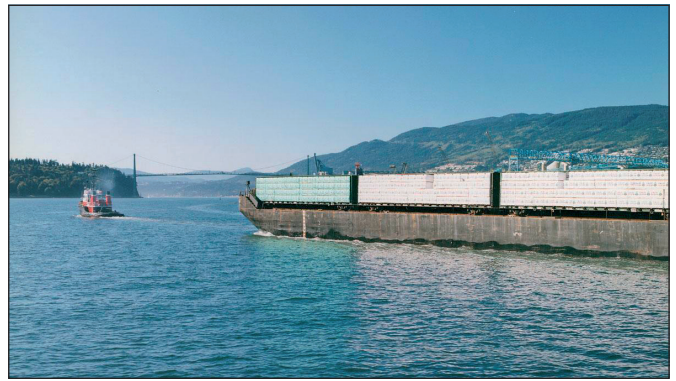
Figure 7: Railcar transportation by tug and barge; common between Vancouver and Vancouver Island.
