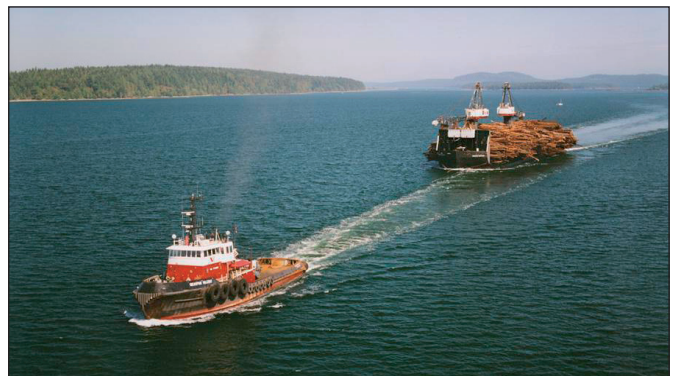
Figure 9: Self loading/self-dumping barges are used to transport logs from remote coastal areas to sorting grounds close to mill sites.
