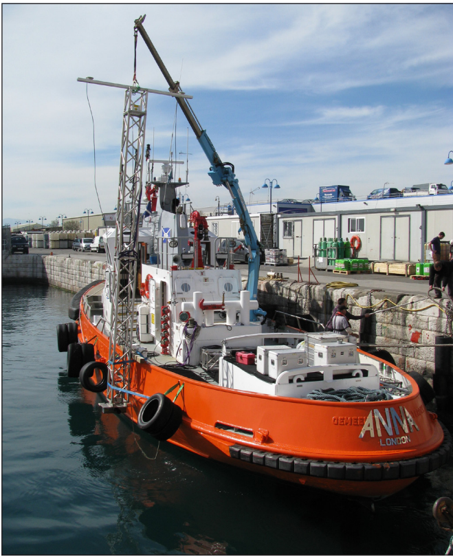
Figure 6: ISHAPS multibeam deployment system on the tug Anna .
