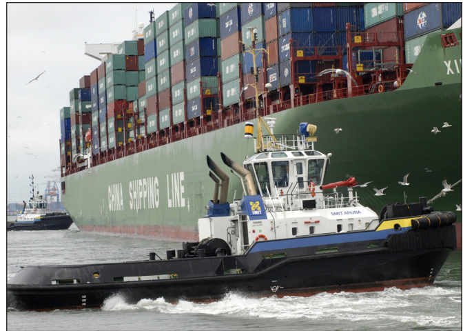
Figure 5: ASD Tug 2810 operating at a ship's side.
