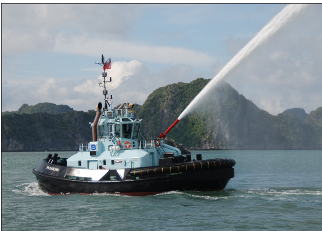
Figure 24: Heavy sausage, W and D fenders on bow, shoulders and sides.
