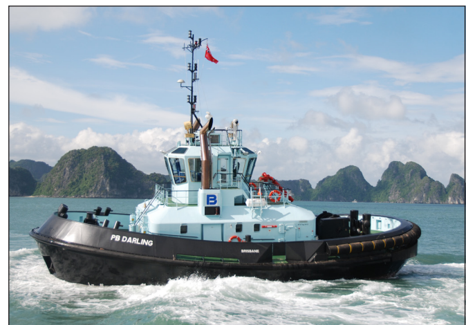
Figure 11: Compact ASD and ATD Tugs have high side thrust.
