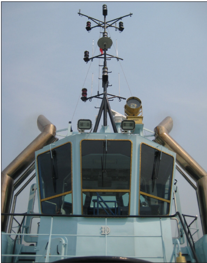
Figure 26: Large windows and shaped superstructure for optimal view.
