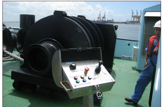
Figure 25: The winch is remote-controlled from the wheelhouse as well as local control on the main deck.
