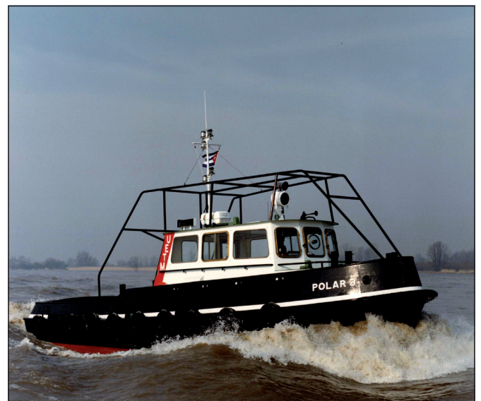
Figure 2: Stan Tug1 – standard compact tug built in 1970 with 700hp.
