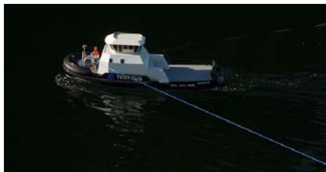
Figure 3: Auto position escort winch system.
