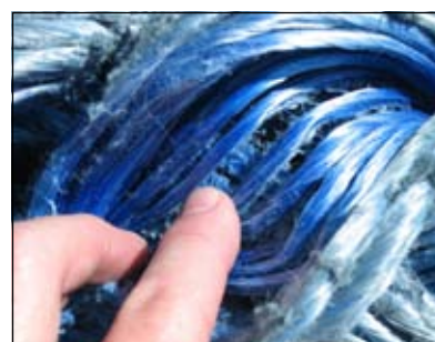
Figure 7(a): Internal wear on a standard 12-strand pendant.
