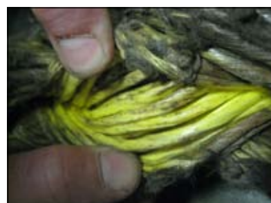
Figure 7(b): Reduced internal wear on a 12-strand pendant with improved coating.
