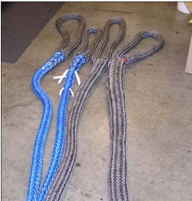
Figure 2: Towlines with eye and body braided chafe gear.
