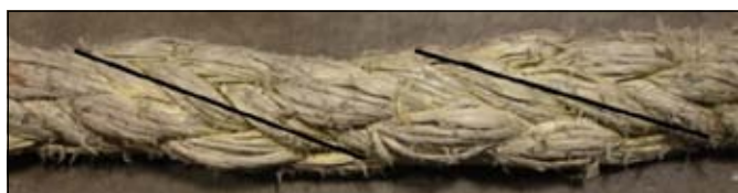
Figure 9: Twist introduced in an HMPE pendant.
