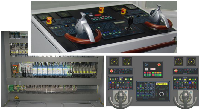
Figure 3: Standard panel, modern compact switchboard with bus control, panel layout with Masterstick.
