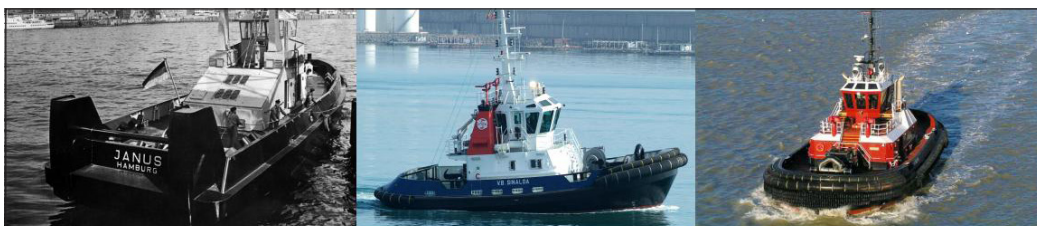
Figure 1, from left, Janus , L: 24m, B: 8.50m, 2x 360kW, BP: 12t; Sinalda , L: 33m, B: 11m, 2x 1,850kW, BP: 65t; Wesley , L: 30m, B: 12m, 2x 2,350kW, BP 75t.
