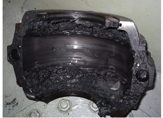
Figure 30: Overheated grease in under-loaded high-speed application.
