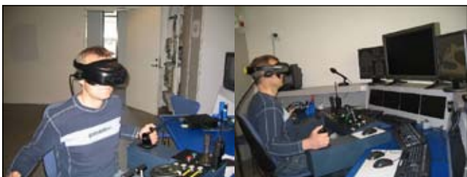
Figure 2: The Visette45 3D lightweight HMD with transparent stereoscopic projector system.
