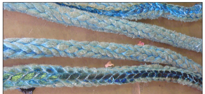
Figures 1 and 2: Section of 64mm AmSteel Blue damaged because it was not secured to the winch drum or bedded in.
