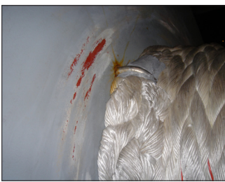
Figure 5: U-bolt fixing tow rope to cheek of drum.
