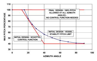
Figure 4 Pitch Control Function to Limit Athwartship Thrust
