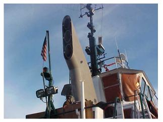
Figure 7 New Foss Stack – Expanded Profile with Integrated 3<sup>rd</sup> Engine Exhaust
