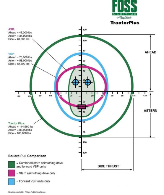
Figure 11 TractorPlus Bollard Pull Characteristics
