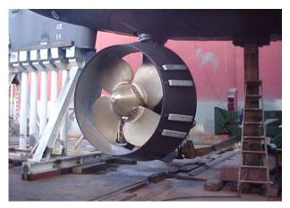
Figure 9 New ASD Unit (with skeg support fixture shown on the left)
