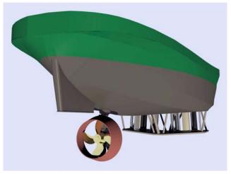
Figure 3 Underbody after Modification
