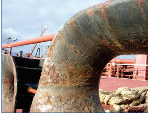
Rust damaged chock typical of crude tankers.
