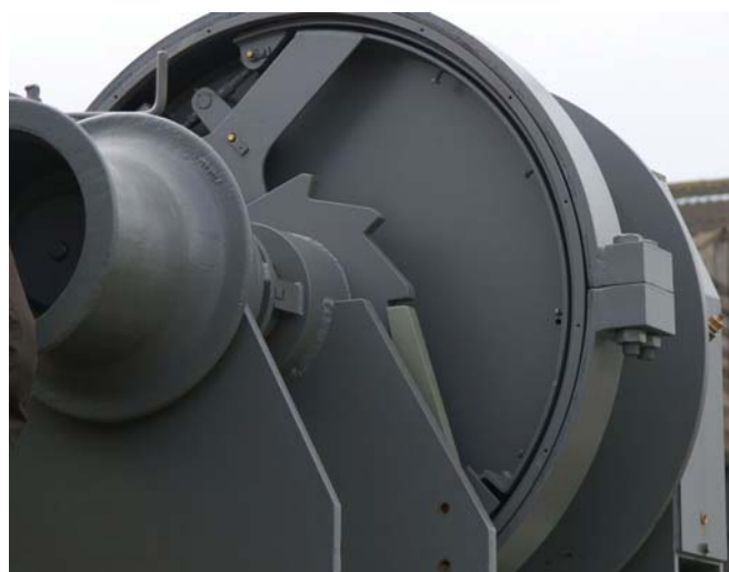
Fig. 10 : Installed ratchet on SafeWinch
