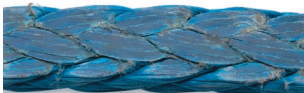
Rope exhibits fiber-set from compression. A slight sheen is visible. This is not a permanent characteristic and can be eliminated by flexing the rope. This condition should not be confused with glazed or melted fiber.
