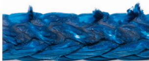
Damage depicted at left caused by excessive heat which melted and fused the fibers. This area will be extremely stiff. Unlike fiber compression, melting damage cannot be mitigated by flexing the rope. Melted areas must be cut out and rope respliced or the rope must be retired.
