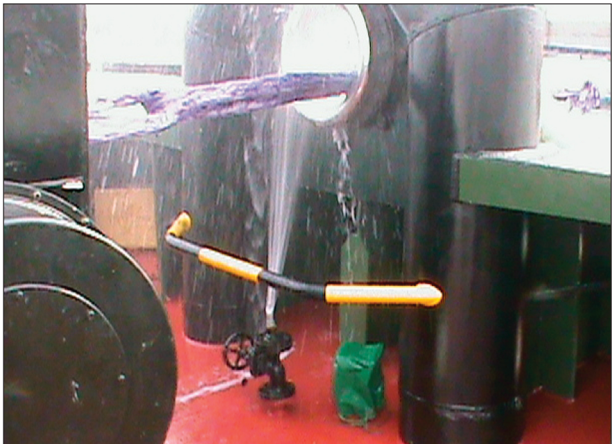
Water Cooling of the hawser on Monterrey . Photo courtesy of Barry Griffin.
