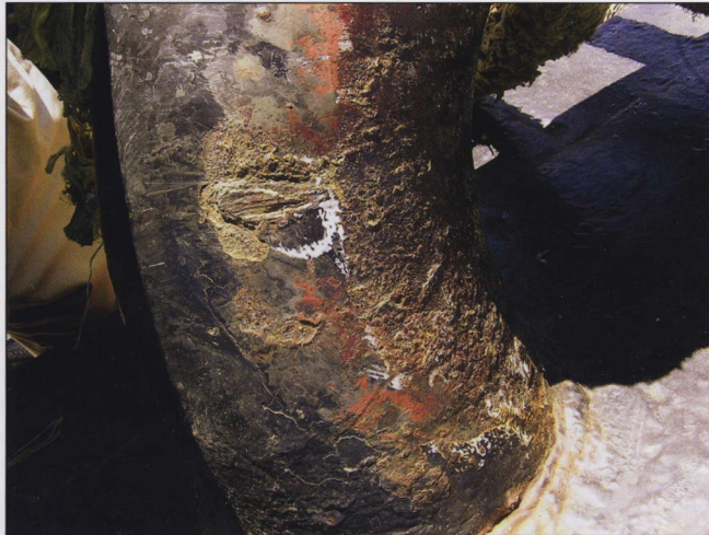
A severely abraded bullnose on a tugboat. Photo courtesy of Samson.
