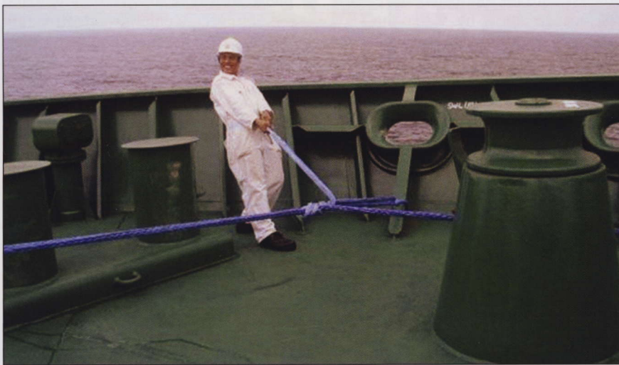
A crewmember adds back tension during the installation of rope onto a winch. Photo courtesy of Samson.
