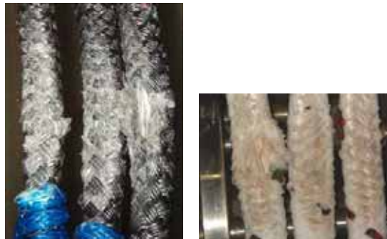
Fig. 15. Visual comparison of the Dyneema® fiber jacket (left) and DPX (right) showed similar wear.
