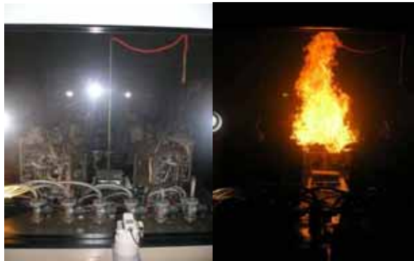
Fig. 7. Flame chamber at Teijin Aramid Inc., to expose rope directly to fire
