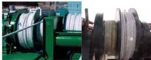
Fig. 17. DPX-75 new (left) vs. 6 months in service (right)
