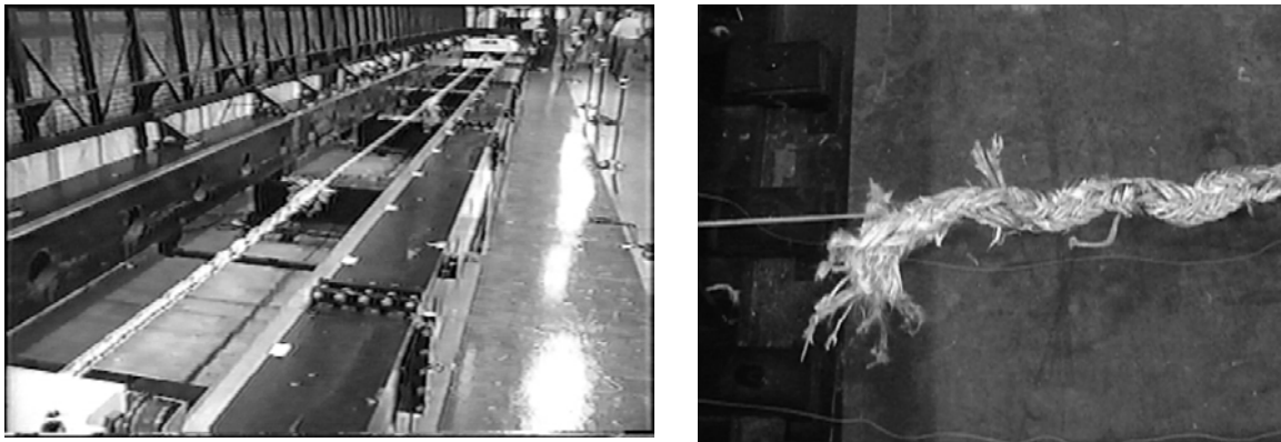
Fig. 4 Rope does not recoil after the 1st break, held together by the stretchy component. The picture in the right shows a close up of the intact stretchy component.
