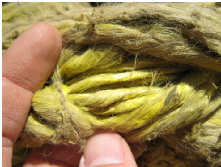
Figure 6. Comparing internal and external yarn condition. [4]
