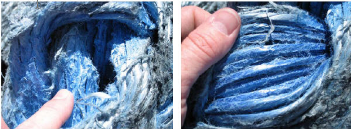
Figure 16. Tug D: Abrasion without chafe protection. [4]
