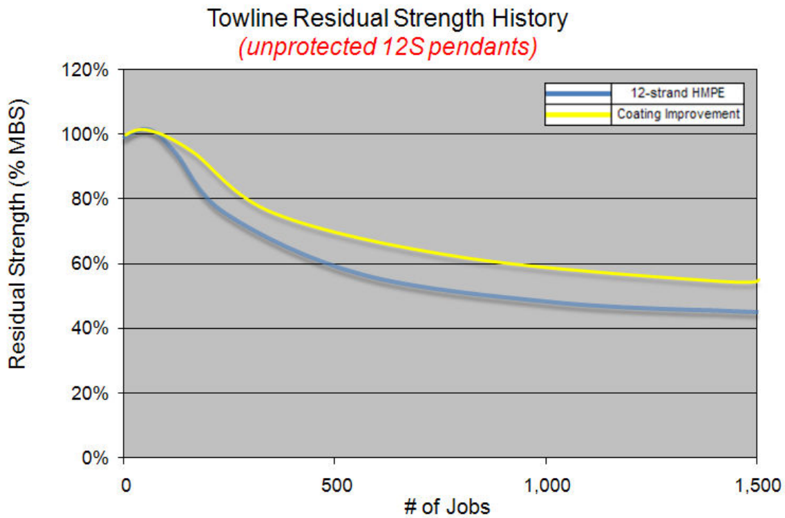
Figure 18. Residual Strength Comparison (coating development).
