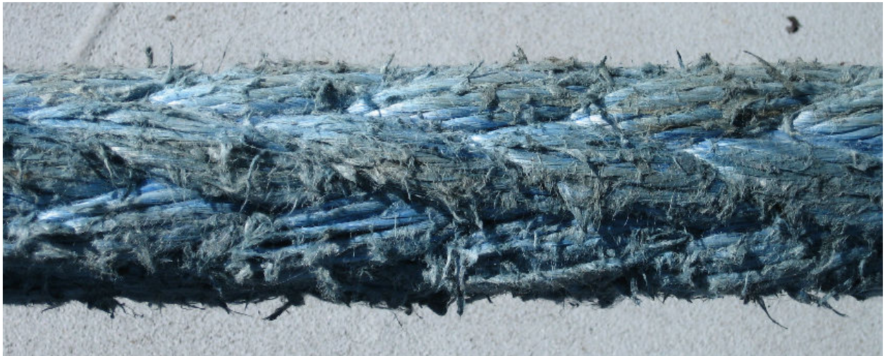
Figure 12. Tug C pendant with chafe protection. This rope has moderate to heavy abrasion damage. [4]
