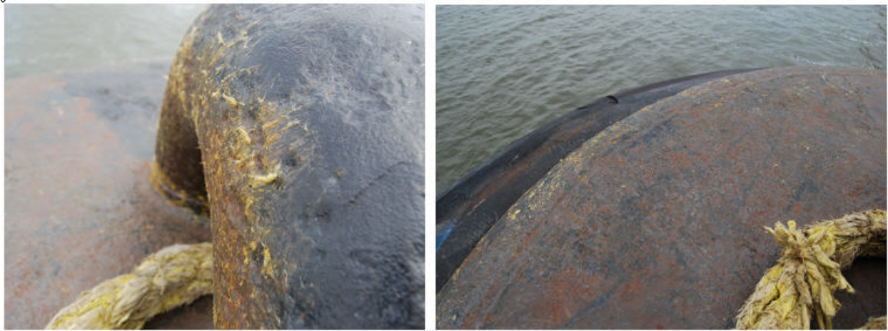
Figure 3. Bull-nose contact surfaces. Rough surfaces cause heavy surface abrasion. [4]
