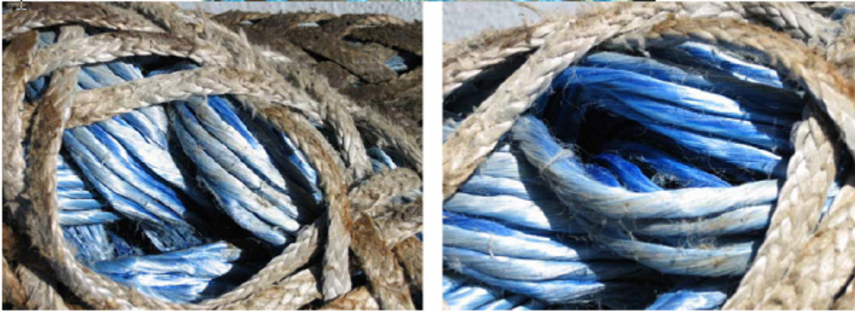
Figure 15. Tug C: Abrasion with chafe protection. [4]
