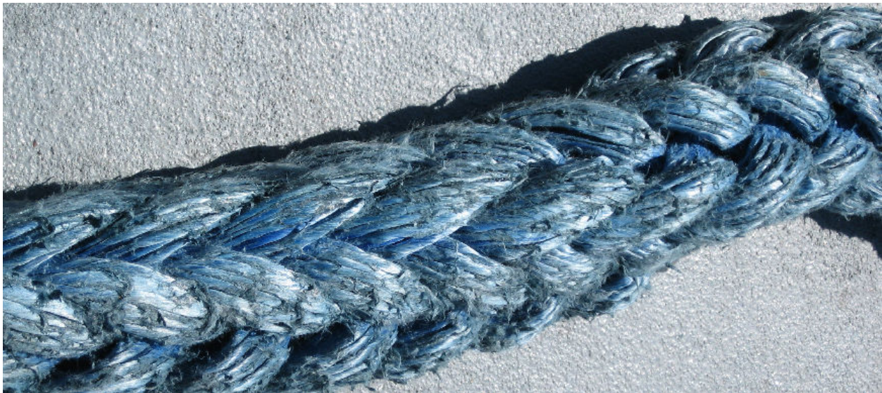
Figure 10 Example of moderate external abrasion. [4]
