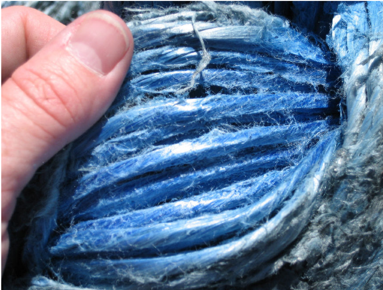
Figure 11. Example of heavy internal abrasion. [4]
