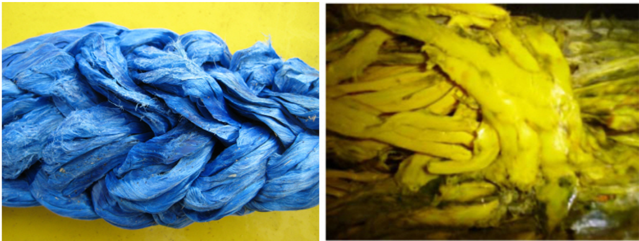
Figure 7. Melted and fused fiber damage. [4]
