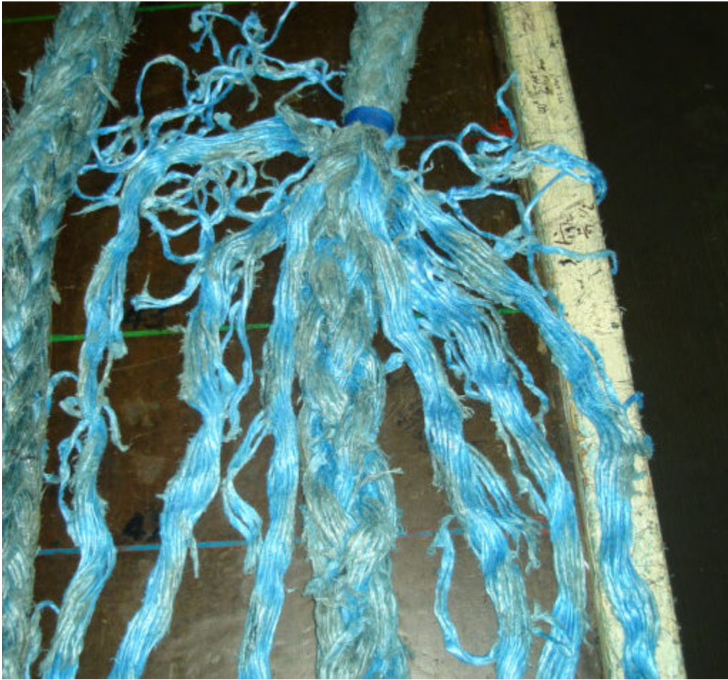
Figure 14. Tug D pendant with cut strands. [4]
