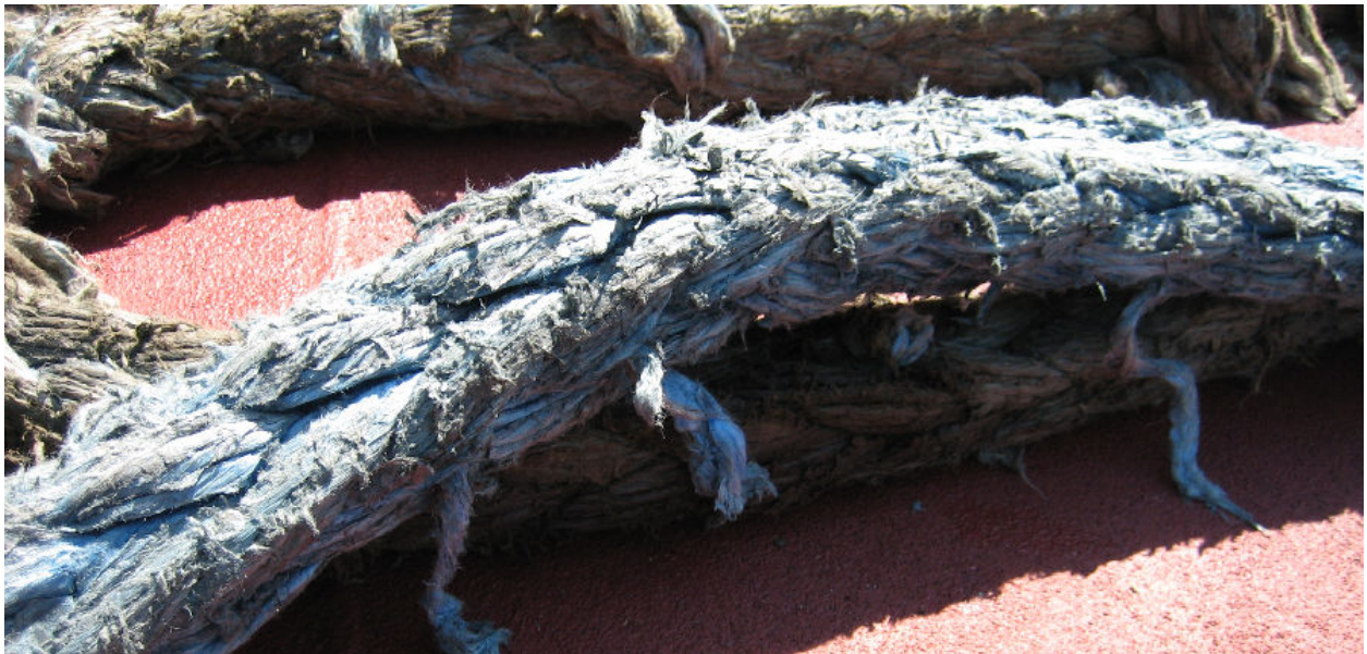
Figure 13. Tug D pendant without chafe protection. This rope has extreme abrasion damage with cut strands. [4]
