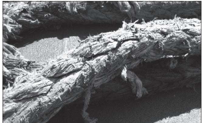
Figure 13: Tug D pendant (extreme abrasion with cut strands) - without chafe protection.
