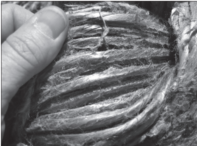
Figure 11: Example of heavy internal abrasion.
