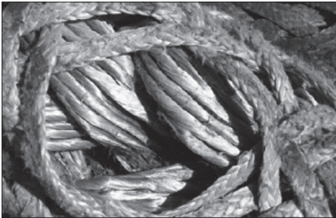
Figures 16a and b: Tug D – abrasion (without chafe protection).
