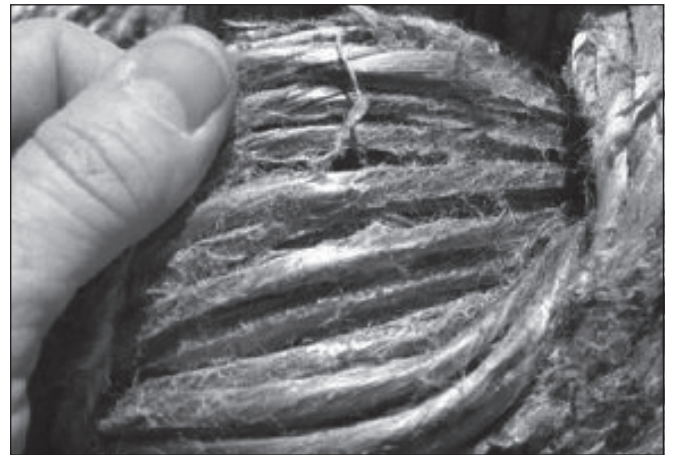
Figures 16a and b: Tug D – abrasion (without chafe protection).
