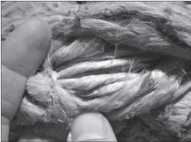
Figure 6: Comparing internal and external yarn condition.
